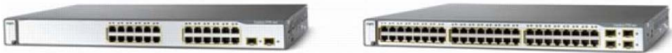
Figure 4: Copper-based LAN workgroup switch akin to a “2x24 splitter and 2x48 splitter”
