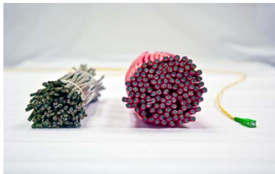
Figure 1: CAT3 cable Kbps capacity, CAT5e cable Mbps capacity and single mode fiber with Tbps capacity
